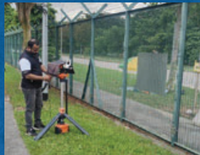
PVAIDS portable camera being redeployed and set up at a new location to mitigate increased intrusion risk from nearby construction.
